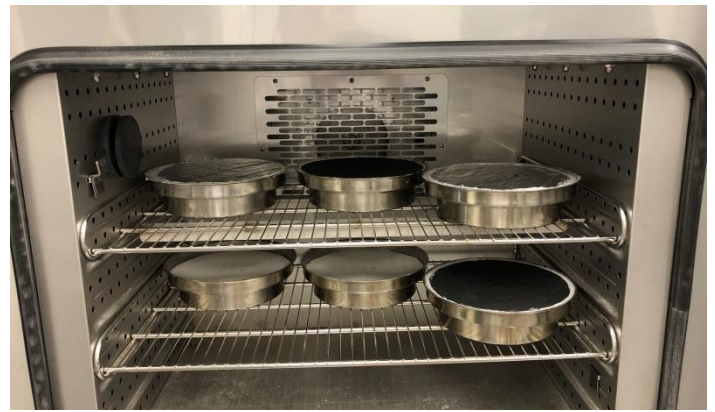
Figure 2 Test cups with specimens in the environmental chamber
